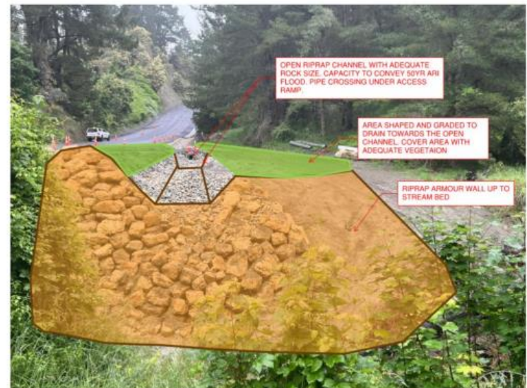
Figure 4-1: Sketches illustrating Option 1 and 2 riprap channel for 50-year ARI peak flows and erosion protection (westbound)
